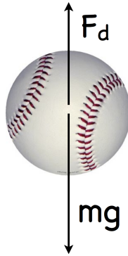
Figure 13.1: Free body diagram for a falling baseball
