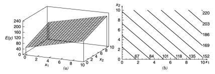
Figure 3.1 (a) The regression plane for the model  $E(y) = 50 + 10x_1 + 7x_2$ . (b) The contour plot.
