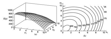
**Figure 3.3** (a) Three-dimensional plot of the regression model  $E(y) = 800 + 10x_1 + 7x_2 - 8.5x_1^2 - 5x_2^2 + 4x_1x_2$ , (b) The contour plot.
