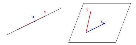
In the first case (colinear), the two vectors are said to be **linearly dependent** (because  $\mathbf{v} = c\mathbf{u}$  for some number c), while in the second case, the two vectors are said to be **linearly independent** ( $\mathbf{v} \neq c\mathbf{u}$  for any c).
