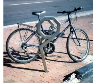
Possible alternatives to the inverted-U bike rack include the simple post-and-ring style (left), or a custom artistic rack (middle) or the abstract rack (right). All styles allow the bicycle to be secured by the frame with a U-lock.
