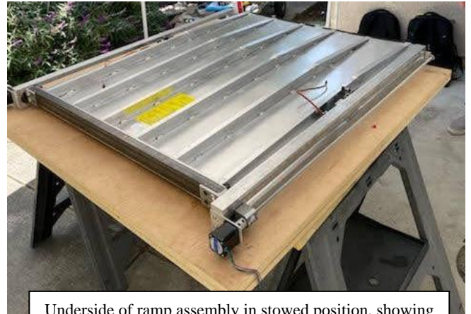
Underside of ramp assembly in stowed position, showing important electronic and mechanical components attached to the fixture that mocks the shuttle chassis.
