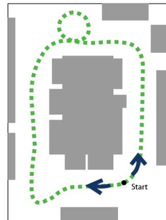
Figure 6. The test track layout in the indoor lab with obstacles marked with solid sections and the test track marked with a dotted line.
