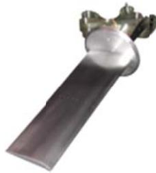
**Figure 3.3 - Clark Y-14 Airfoil (AEROLAB, 2007)**
