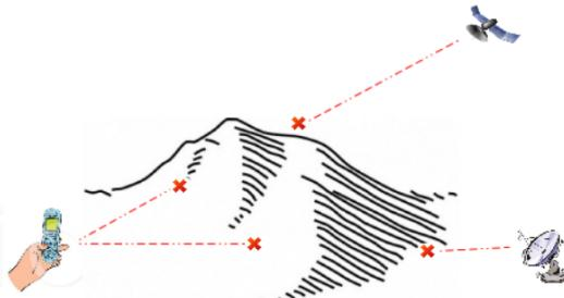
Figure 1: Line-of-Sight obstructed by terrain.
