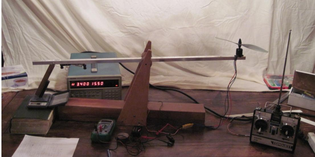
**Image 5:** Lever apparatus to measure thrust. The upwards thrust from the motor/rotor on the right side is converted into a downwards force to the digital scale on the left side.
