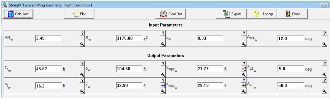
Figure 15. Straight tapered wing geometry
