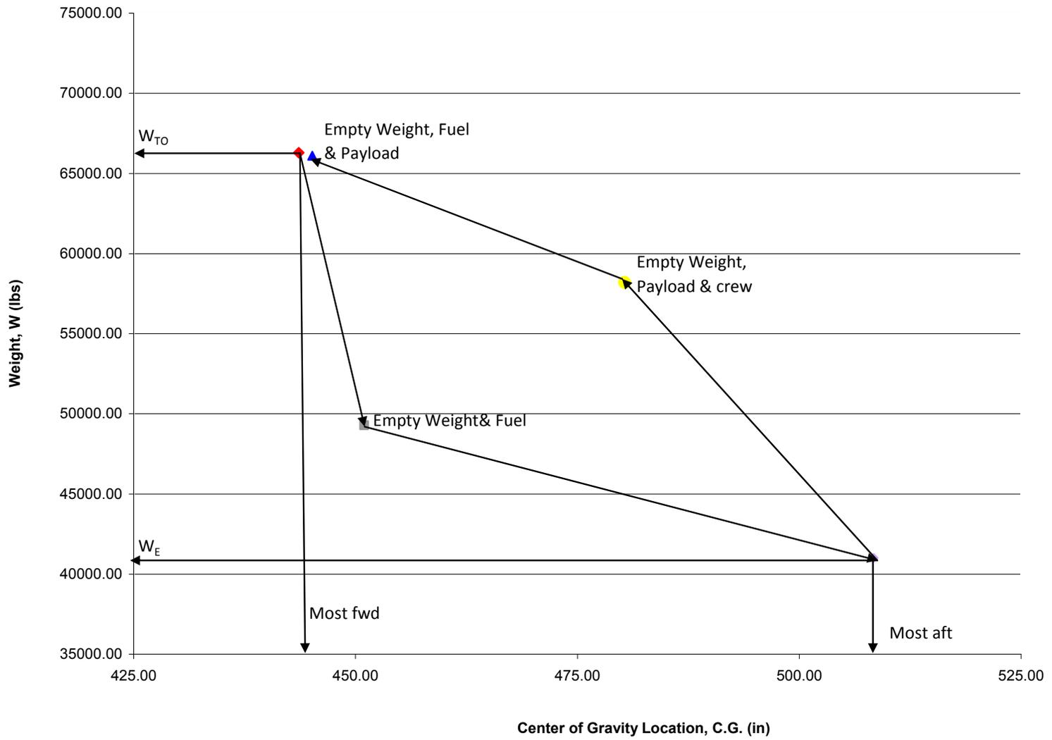
Figure 36. Center of Gravity excursion diagram
