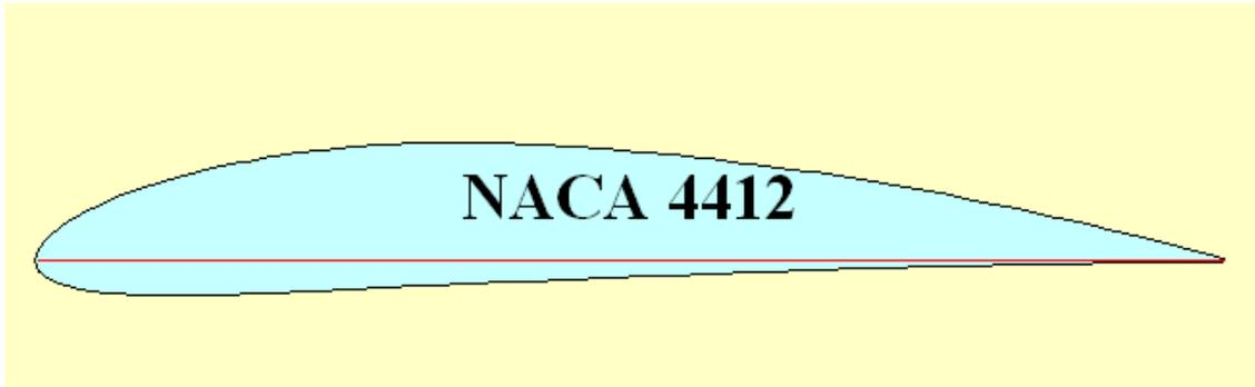
Figure 21. Shape of NACA 4412 airfoil
