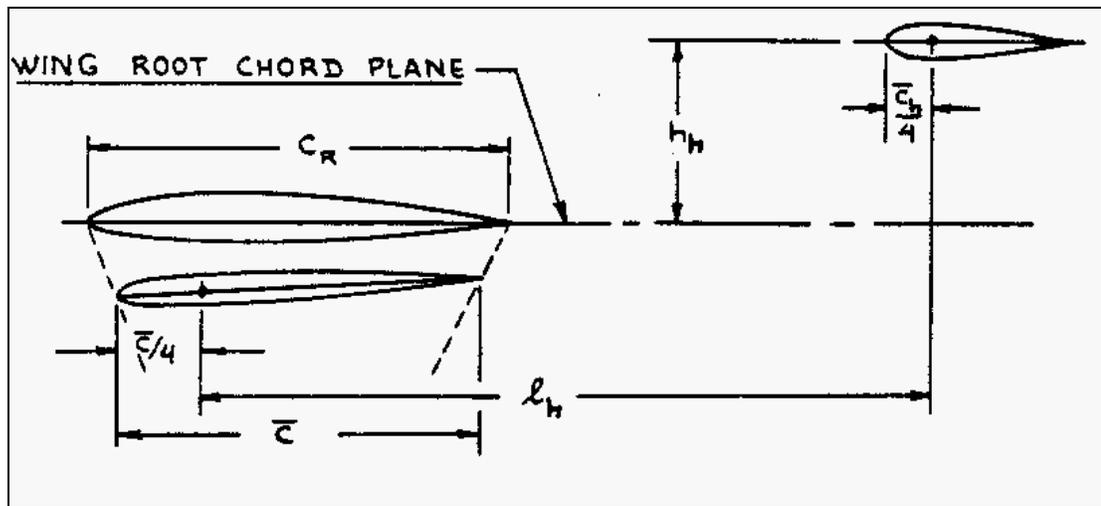
Figure 38. Geometric parameters for horizontal tail location
