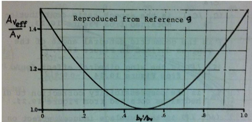
Figure 41. Effective value of vertical tail aspect ratio
