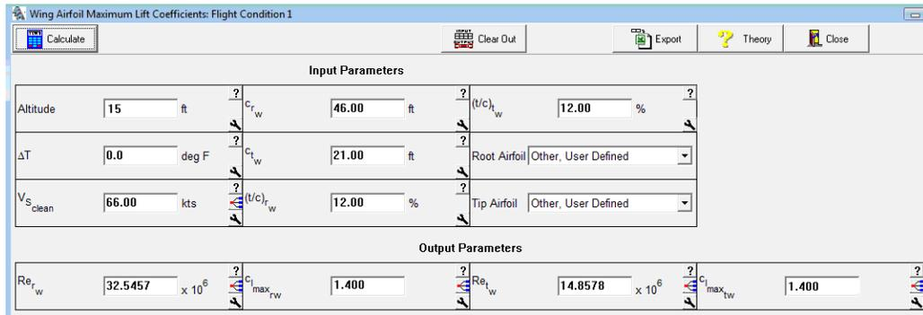
Figure 18. Calculation of lift coefficient using AAA program
