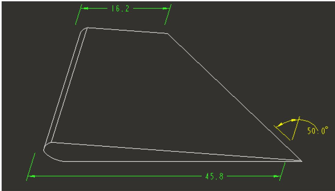
Figure 19. Geometry of a wing
