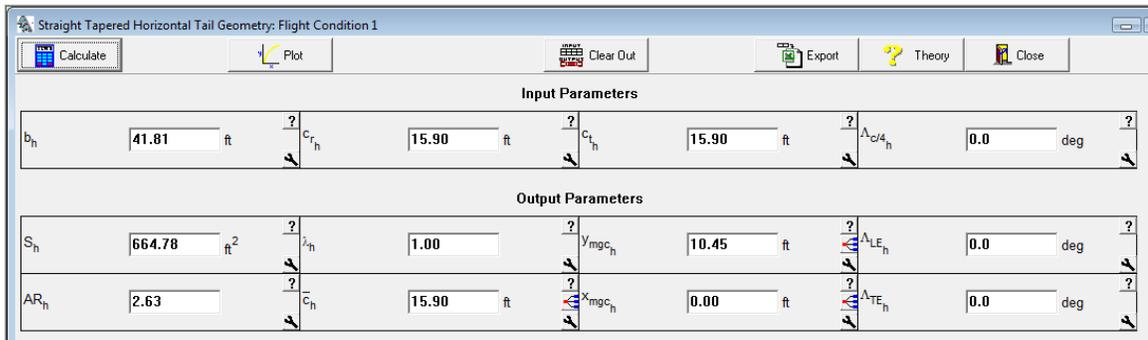
Figure 25. Horizontal tail geometry untapered using AAA
