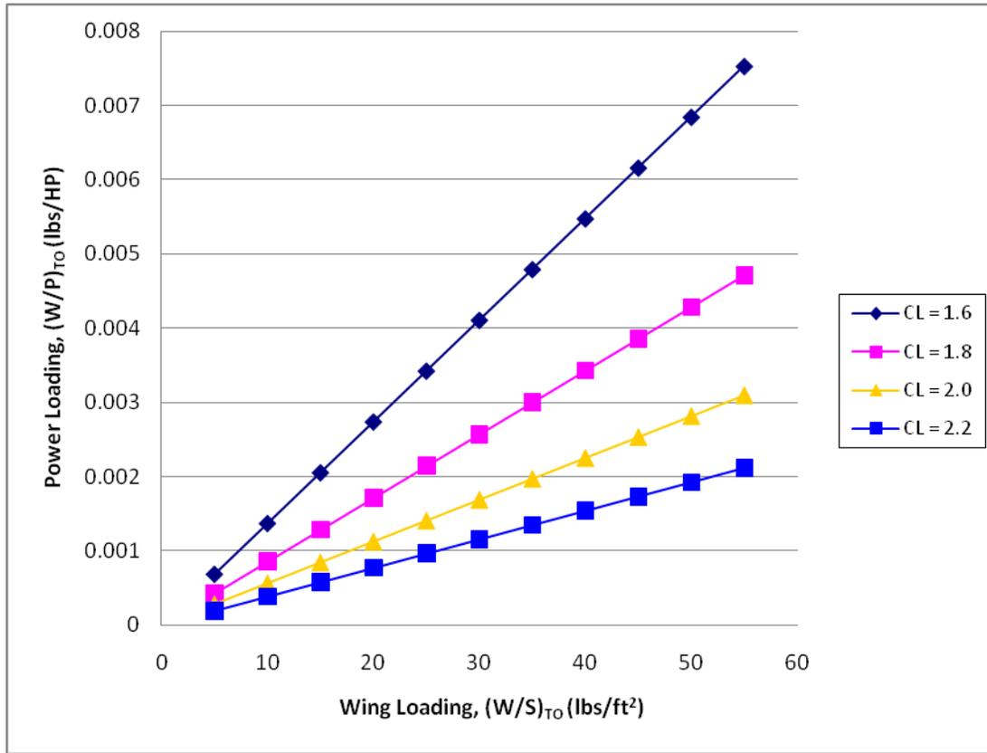
Figure 8. Power loading vs Wing loading as a function of varied lift coefficient
