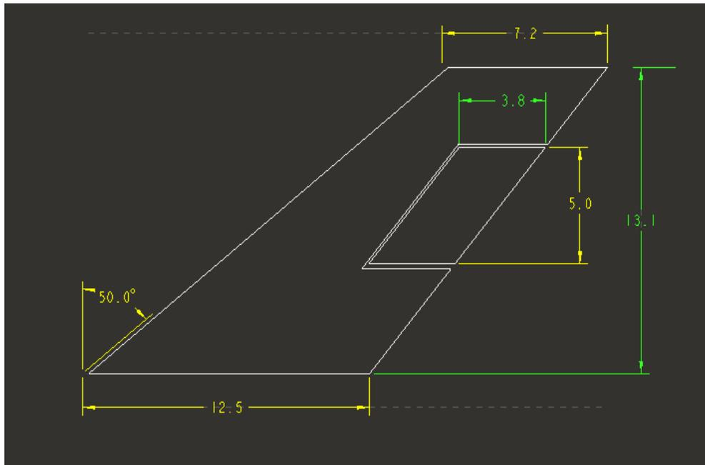
Figure 30. Geometry of a vertical stabilizer
