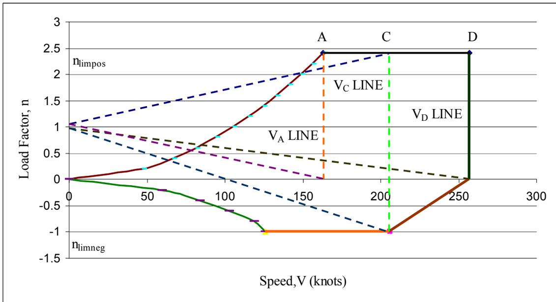
Figure 49. V-n Diagram
