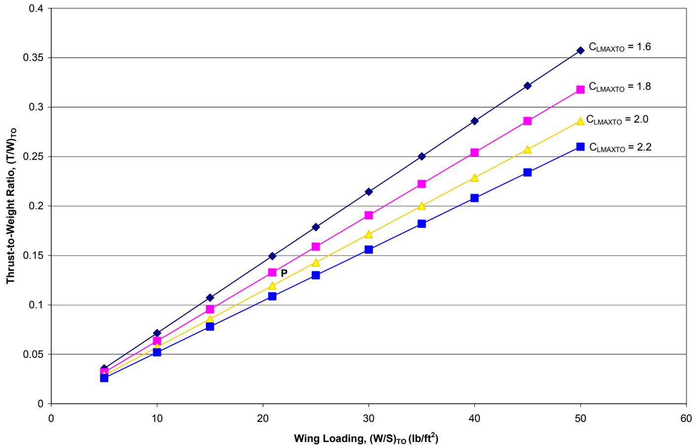
Figure 7. Thrust-to-weight ratio vs Wing loading as a function of varied lift coefficient
