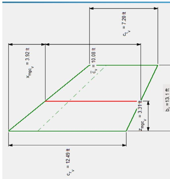
Figure 27. Vertical tail planform using AAA
