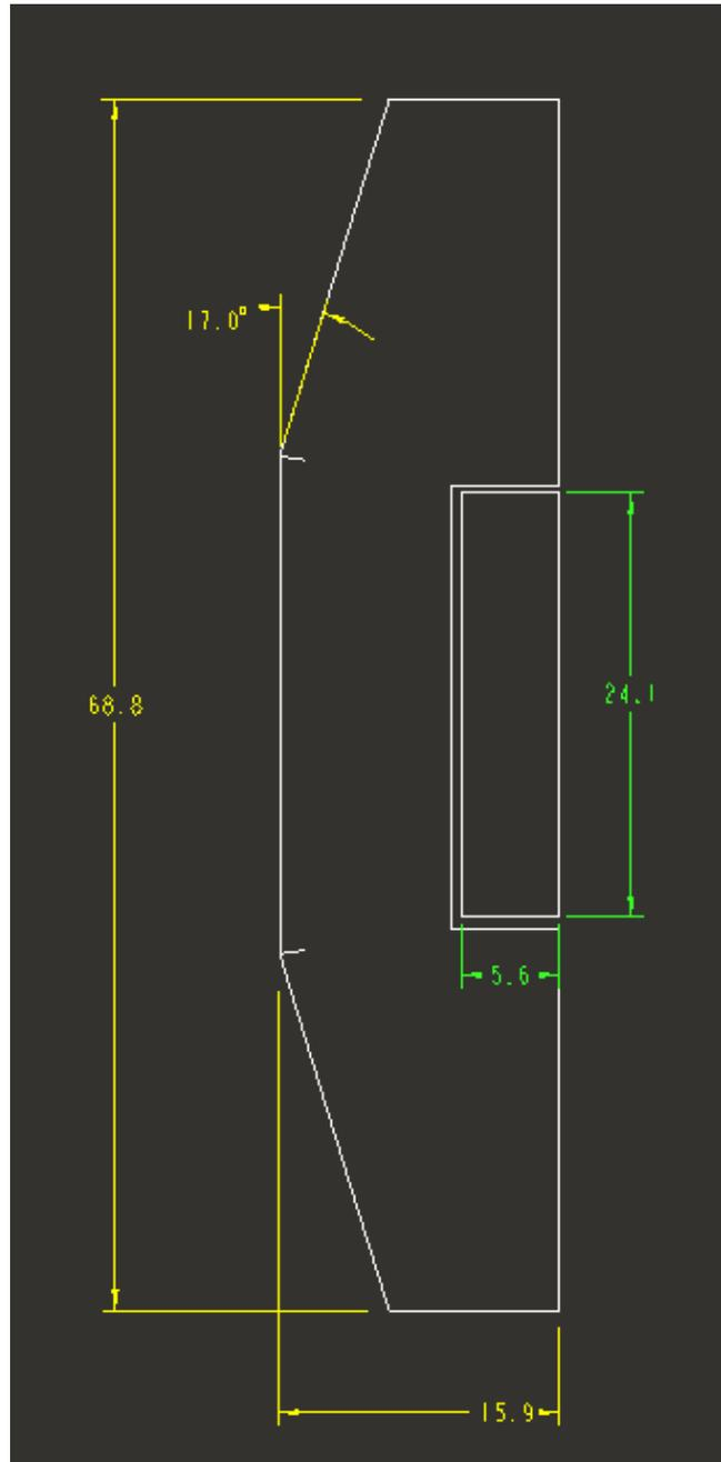
Figure 33. Geometry of a horizontal stabilizer
