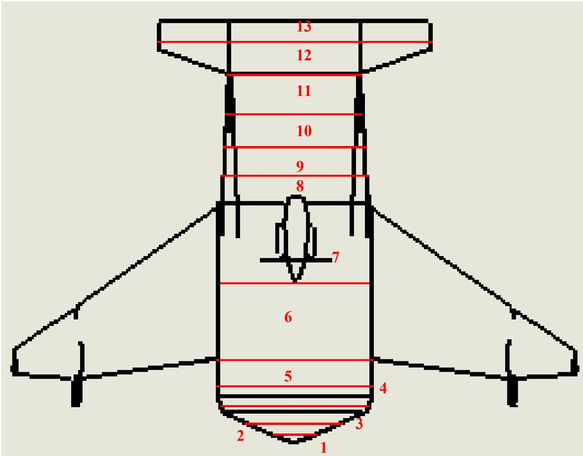
Figure 39. Layout for computing fuselage and contribution to airplane aerodynamic center location
