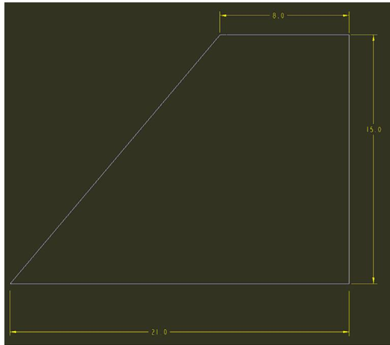
Figure 20. Geometry of a winglet
