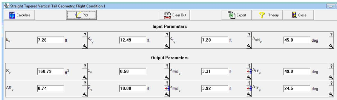
Figure 26. Vertical tail geometry using AAA
