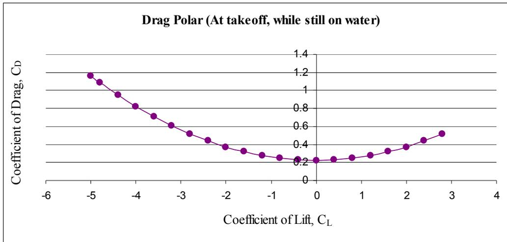
Figure 46 Drag Polar (At takeoff, while still on water)
