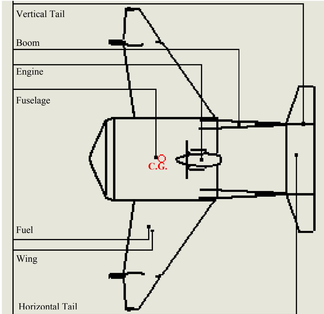
Figure 34. Location of centre of gravity in X-direction
