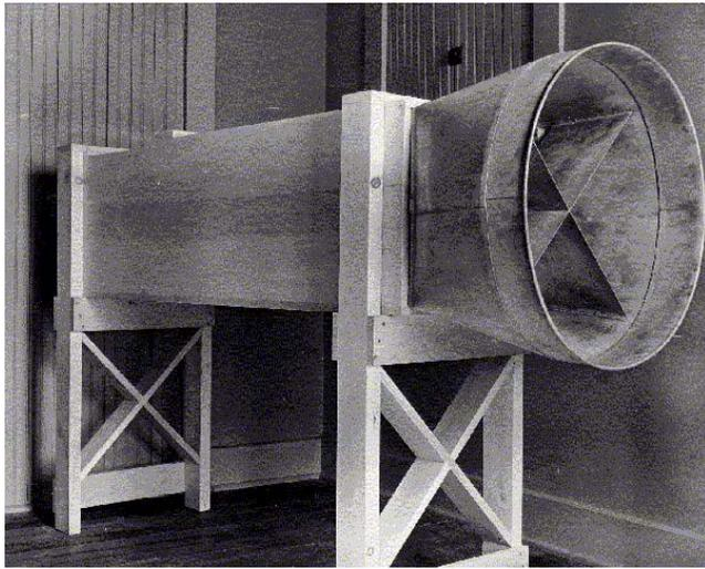
Figure 3. The Wright brothers wind tunnel, used to obtain their wing and airfoil data.
