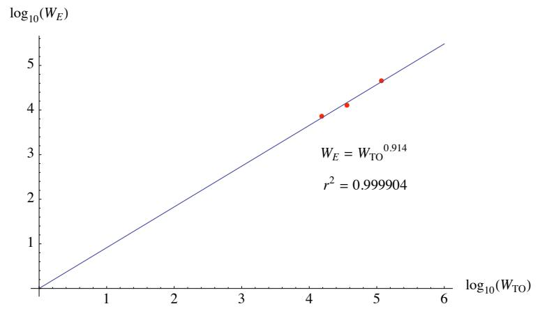
**Figure 10. Weight trend for modern airships.**
