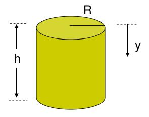
A cylinder with radius R and a non-uniform mass density  $\rho(y) = 4 + 3y$ . (All quantities are in SI units).
