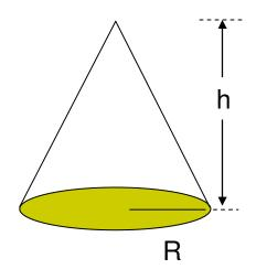
A regular symmetrical cone with circular base of radius R has a volume of  $(1/3)\pi R^2h$ .
