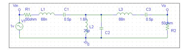
Fig. 1 The circuit of three order bandpass by calculating values
