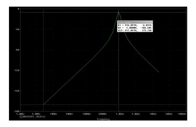
Fig.2 The Pspice waveform of three order bandpass filter by calculating values
