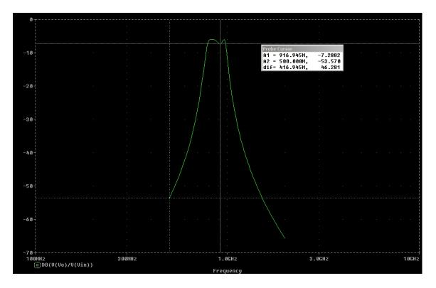
Fig. 3 The waveform of three order bandpass filter by real components
