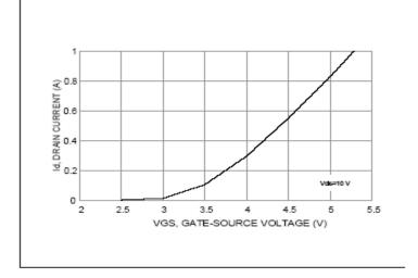
Figure 3: Vd Vs Vg curve for PD57006
