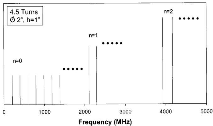
Fig. 3. Spectrum for  $n = 0, 1,$  and  $2$  modes of a helical resonator approximated by the sheath model.
