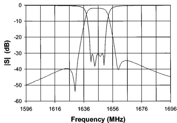
Fig. 5. Measured quasi-elliptical response of a dual-mode helical resonator loaded cavity filter (four pole 10-MHz bandwidth, 1.8-dB insertion loss, realized unloaded  $Q$  of 1400).
