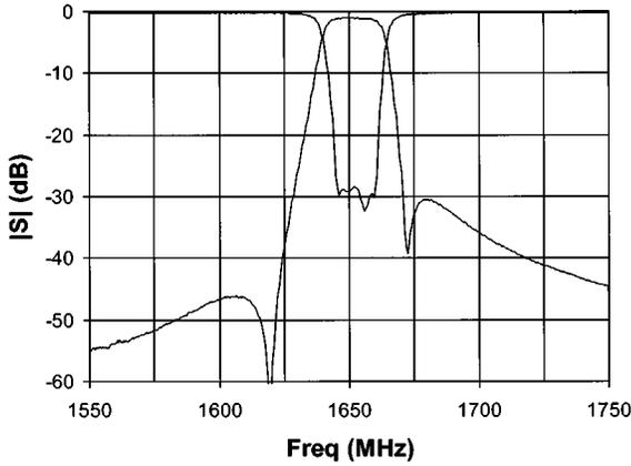
Fig. 6. Measured response of the same filter in Fig. 4 with silver-plated elements and new coupling probes (quasi-elliptical response, 15-MHz bandwidth, 0.96-dB insertion loss, realized unloaded  $Q$  of 1800).
