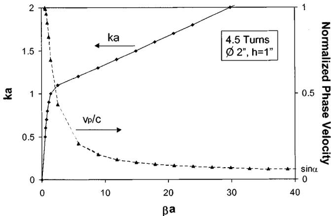
Fig. 1. Dispersion relation and phase velocity of a sheath helix operating at  $n = 1$  mode.
