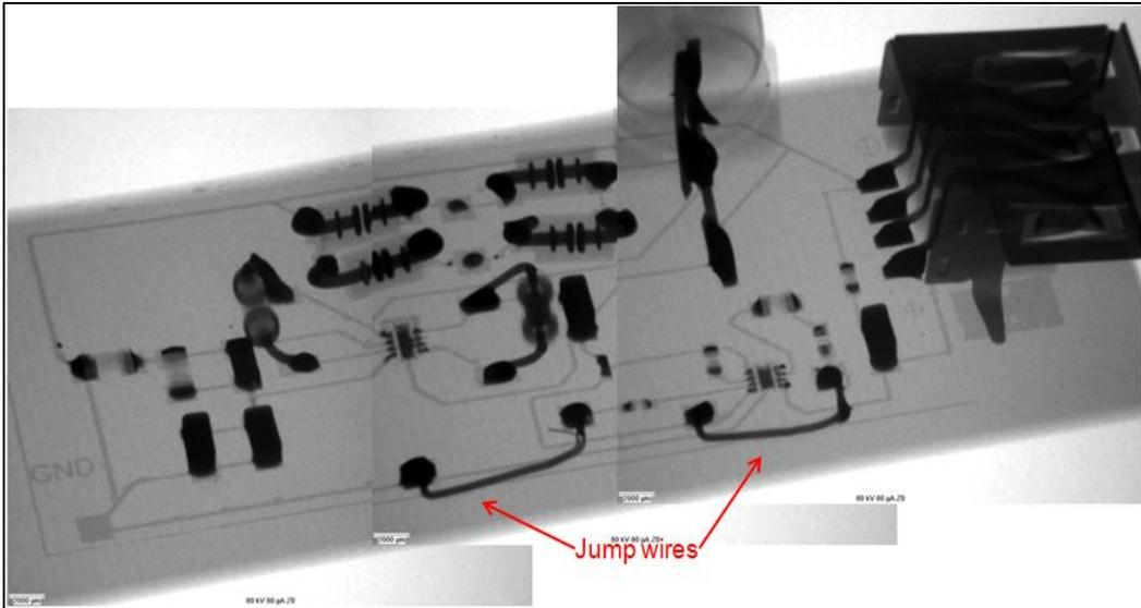
Figure 9: X-ray of PCB. Each part of the board was expected to ensure no shorting had occurred.
