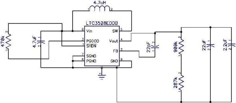
Figure 4: LTC3528 schematic
