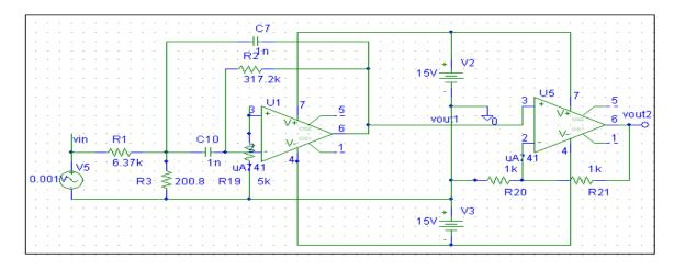
Figure 3.5. PSpice schematic of each band-pass filter.
