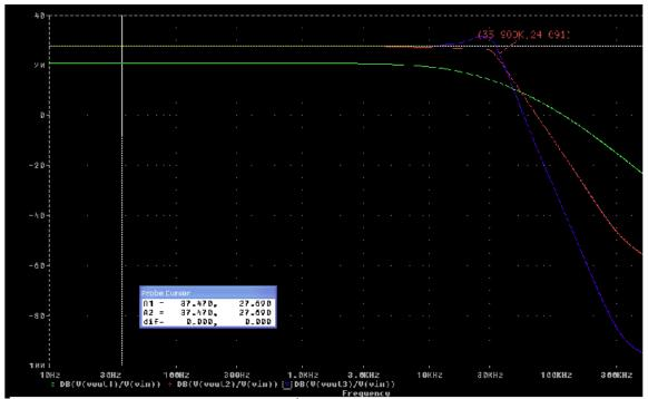
Figure 3.4. Bode plot of 5<sup>th</sup> order Butterworth low-pass filter.
