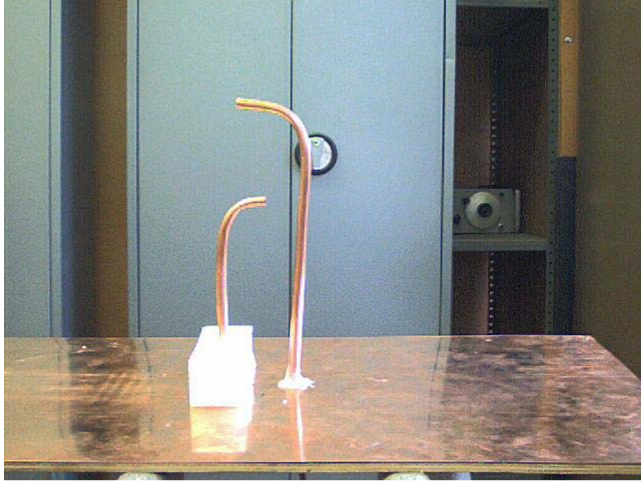
Figure 12: Prototype built using 45° cut tubing, more precise dimensions.
