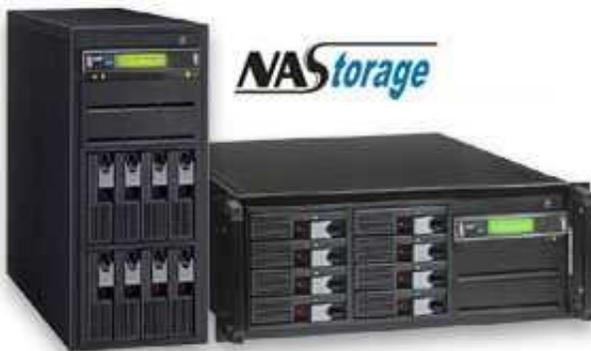
FIGURE 1.4: Network Attached Storage (NAS) devices that are directly connected to the cluster-level switching fabric
