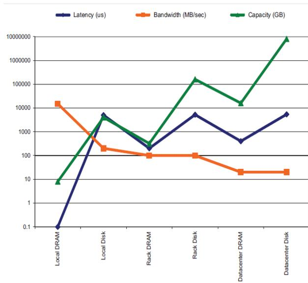
**FIGURE 1.6:** Latency, bandwidth, and capacity of a WSC.
