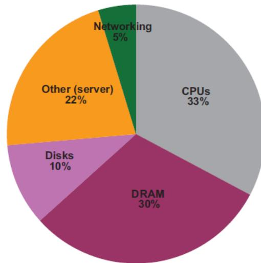
**FIGURE 1.7:** Approximate distribution of peak power usage by hardware subsystem in one of Google’s datacenters (circa 2007).
