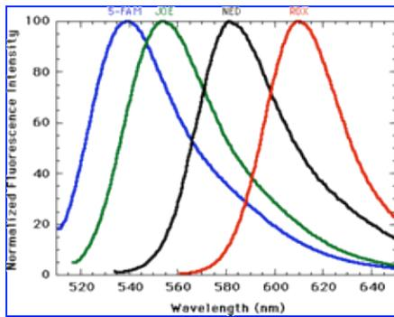
Although the dyes are different colors, their spectra can overlap because the wavelengths that determine color occur simultaneously, not discretely.
