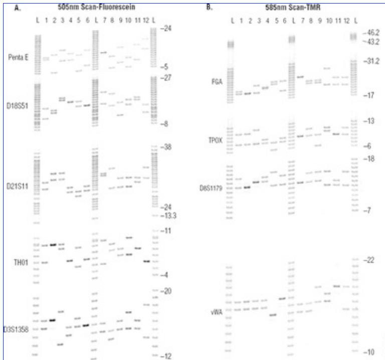
Promega was the first commercial manufacturer in the country to offer a STR multiplex that typed all of the CODIS core loci with a single amplification. The kit, PowerPlex® 16, is a three-dye kit that amplifies 15 STR loci and amelogenin in the following configuration:
