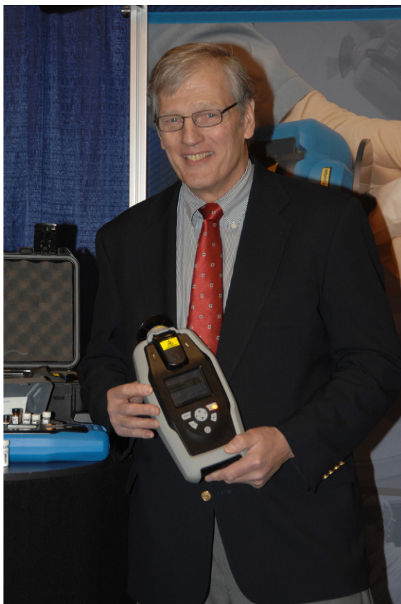
Fig. 5. A portable Raman spectrometer. This device has shown great promise in identifying explosives and polymers using an internal library, and it has potential to be applied to body fluid identification as well. Mixture analysis software can identify components of solid/liquid combinations and aqueous solutions, and it weighs less than 4 lbs. (With kind permission from C&EN and Mitch Jacoby.)
