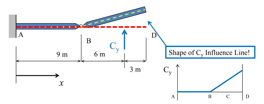
3. The **rigid body** motion of the modified unstable structure is the shape of the influence line for the response quantity.
