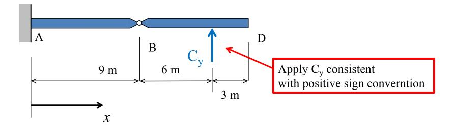
2. Apply the response quantity to the modified unstable structure from Step 1.
