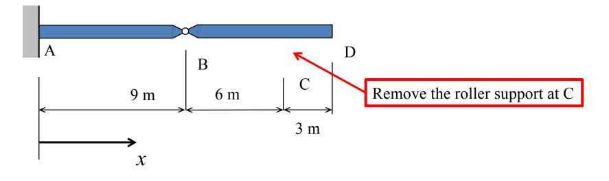
1. Remove the ability for the structure to resist the response quantity (e.g. reaction, internal shear, internal bending moment at a particular point). For a determinate structure this will result in an unstable structure.
