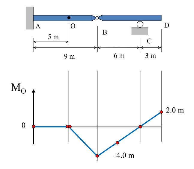
General procedure for the applying the Muller-Breslau principle to find the shape of influence lines
