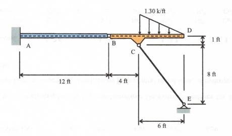
The stable beam shown above is supported by a rigid support at point **A** and a member that is pin connected at points **C** and **E**. The beam has an internal hinge at point **B**.
