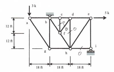
For the pin connected stable truss, subjected to the point loads shown and pin supported at joint **b** and a roller support at joint **i**, calculate the following:
