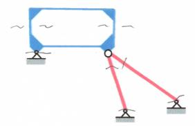
For the structure shown above, subjected to general loading, determine if it is **Determinate**, **Indeterminate**, or **Unstable**.
