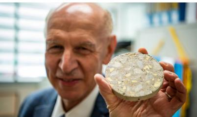
Professor Al-Manasser holds an example of sustainable ductile concrete containing recycled reaction injection molding (RIM) plastic which can reduce brittleness in concrete upon impact with a moving vehicle.
