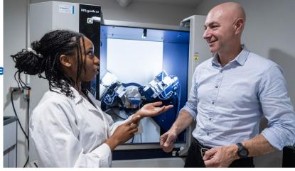
Graduate Student Nalina Johnson and Professor and Moss Landing Marine Laboratories Interim Director Ivano Aiello stand before an x-ray diffractometer used to test and measure estuary soil samples with the results used to improve the decision-making in estuary restoration.
