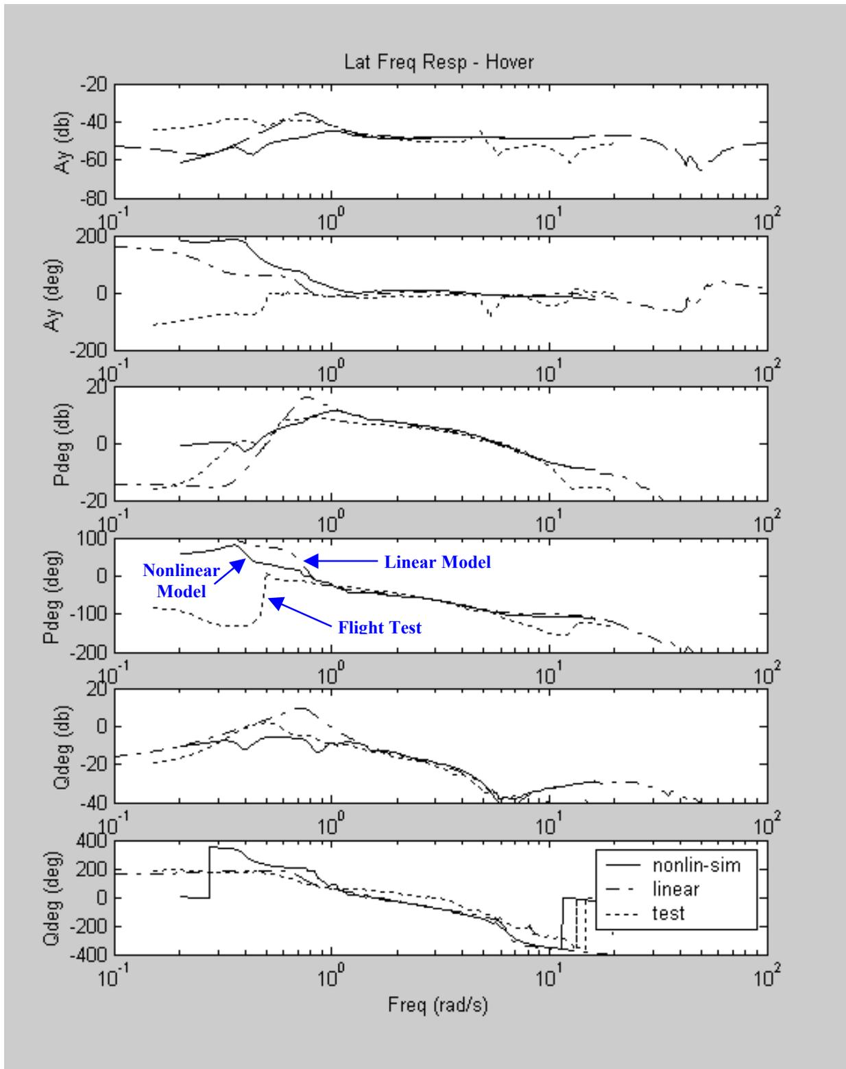
Figure 2 Model Verification and Validation Data: Lateral Acceleration, Roll Rate, and Pitch Rate Responses to Lateral Input
