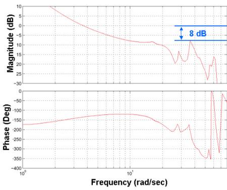
Figure 5 Longitudinal Hover Case ASE Stability
