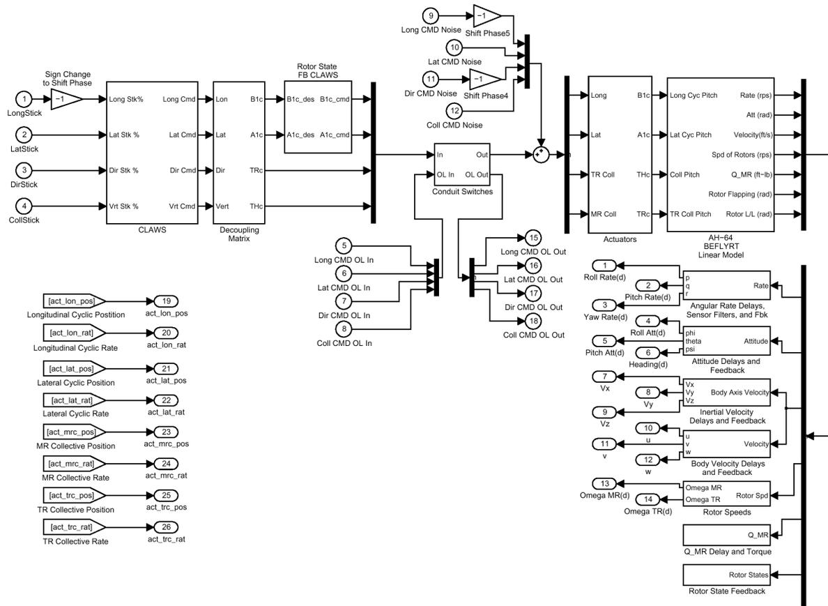
**Figure 3 HFCS Analytical Model Block Diagram**
