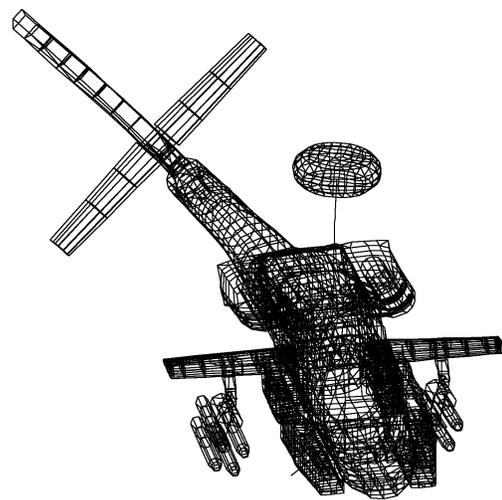
**Figure 1 Exaggerated Motion of 4.5 Hz Lateral Bending/Tailboom Torsional Mode**
