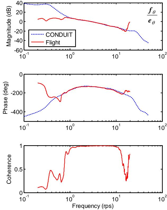
**Figure 5 – Analysis validation, broken-loop response, velocity hold mode ( $f_\theta/e_\theta$ )**
