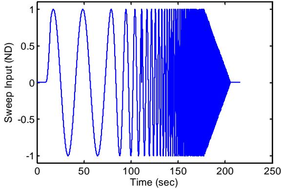
**Figure 4 – Example automated sweep input**
