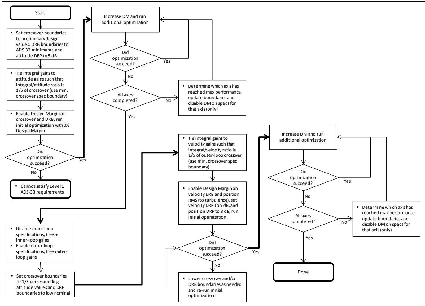
**Figure 9 – Graphical representation of Nested optimization approach**
