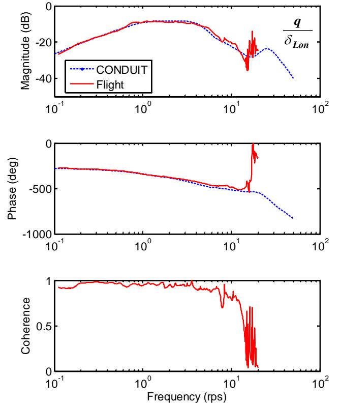
**Figure 7 – Analysis validation, closed-loop response, ( $q/\delta_{Lon}$ )**
