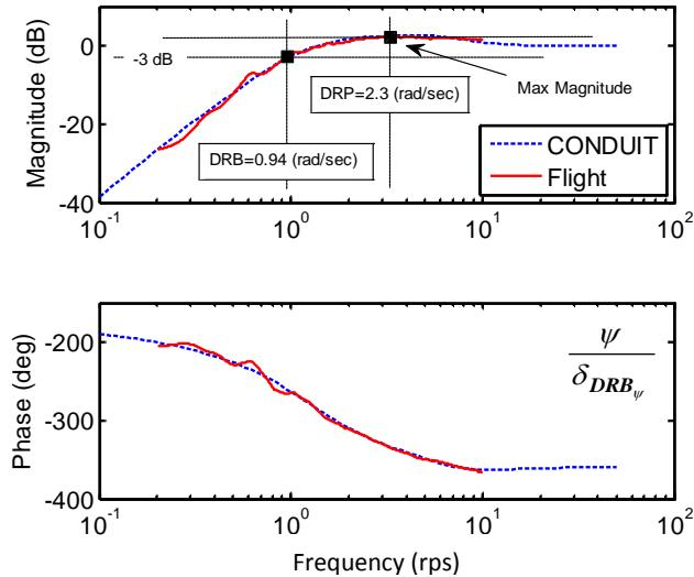
**Figure 6 – Analysis validation, disturbance response, ( $\psi/\delta_{DRB_\psi}$ )**
