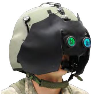
Fig. 4: NVG setup for simulated DVE
