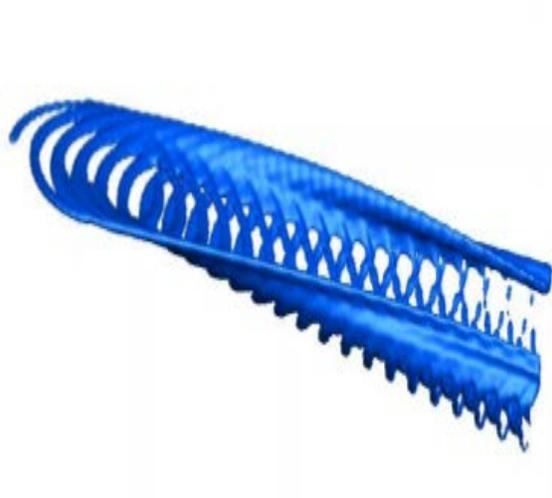
Figure 15: A Snap shoot of rotor wake vorticity iso-surface resulting from thrust based inflow forcing excitation at 80 knots
