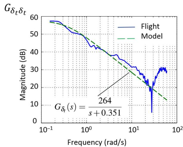
(b) Longitudinal CETA turbulence identification from flight (Ref. 110)
