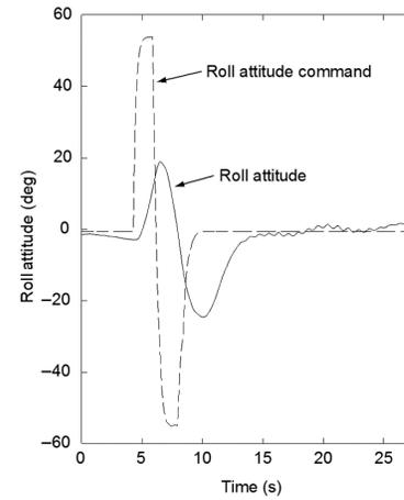
(c) Re-design based on identified delay  $\tau_e = 290$  ms
