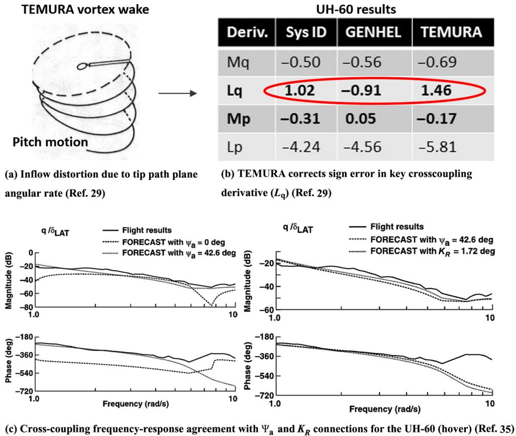
Fig. 11. Wake distortion as the source of cross-coupling sign-error discrepancy.
