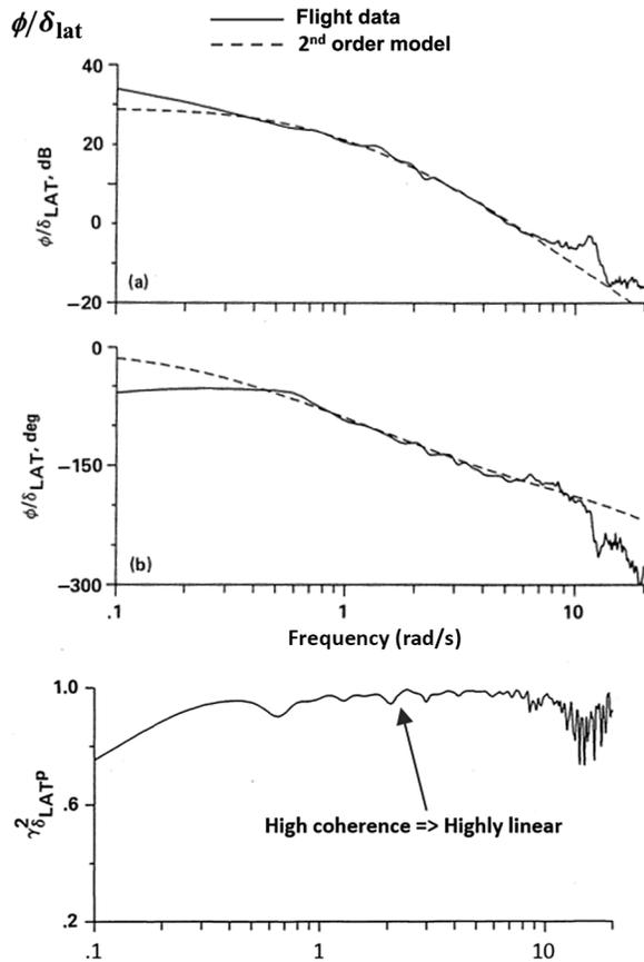
(c) Frequency response and coherence determination with transfer-function identification
