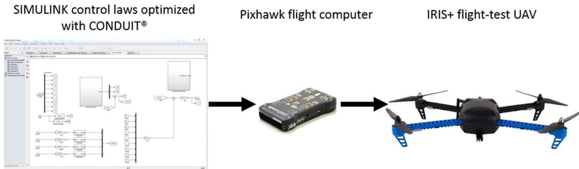
(a) Pictures-to-code process and flight-test platform (Ref. 109)
