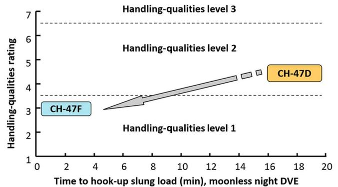
(b) Comparison of time-to-hookup load on a moonless night in operational tests: CH-47F DAFCS vs. CH-47D (data released by U.S. Army DAFCS program office)
