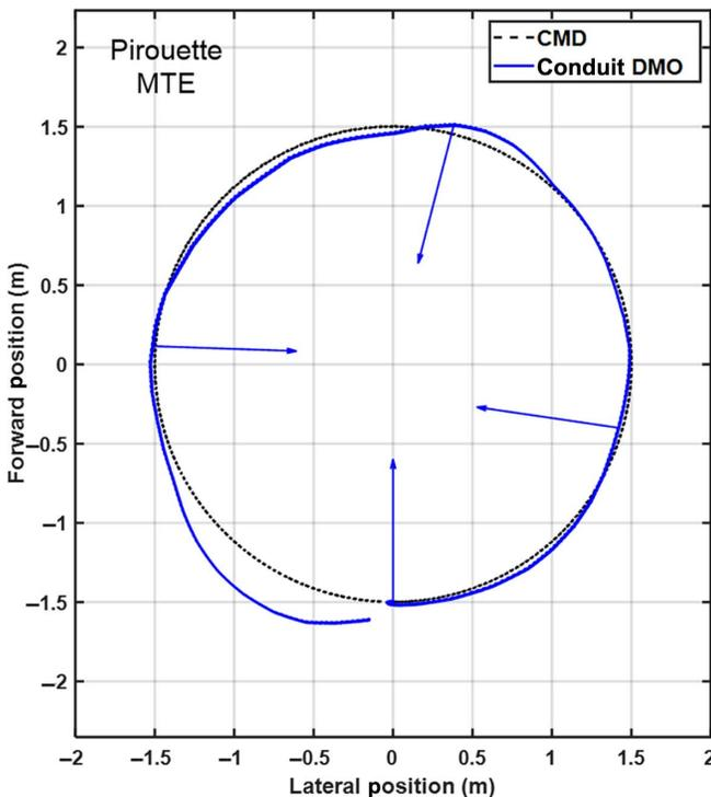
(c) Flight-test results of optimized design (solid line) vs. commanded ground track (dotted line) for Pirouette maneuver
