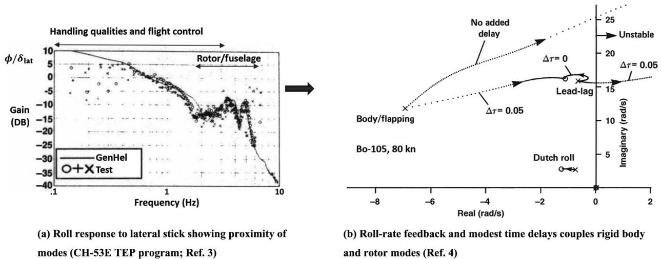
Fig. 3. Overlap and coupling of dynamics modes of rotorcraft.
