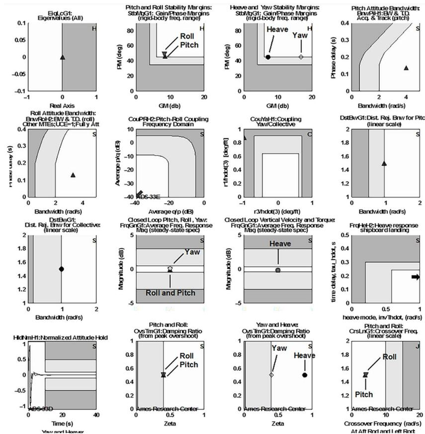
(b) CONDUIT<sup>®</sup> optimization of control laws using system ID LTI model (hover)
