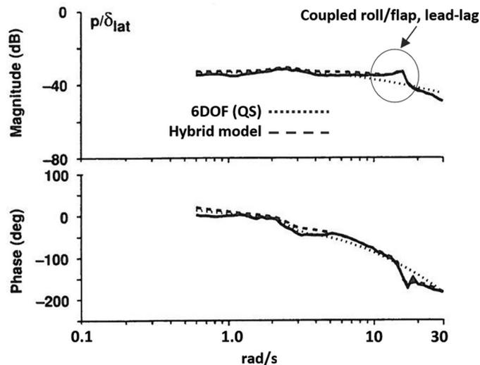
Fig. 16. Bo-105 higher order rotor/fuselage model identification, 80 kt (Ref. 54).
