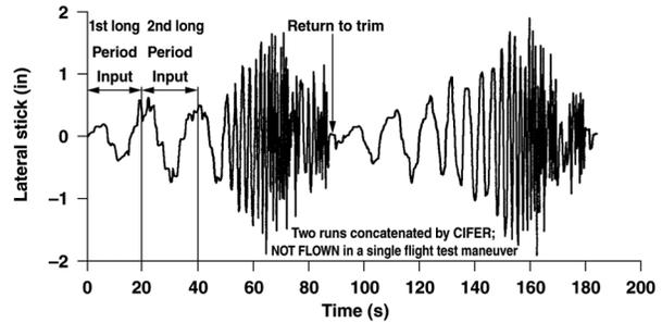
(b) B214ST piloted frequency-sweep test data
