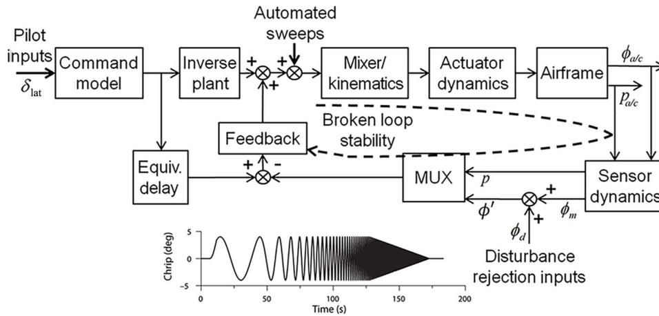
(a) Automated frequency-sweep flight-test method to determine DRB (roll attitude hold)
