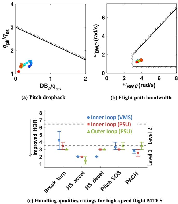
**Fig. 25. Validated adoption of fixed-wing experience and outer loop control to the high-speed regime for generic coaxial-pusher configuration (Ref. 98).**
