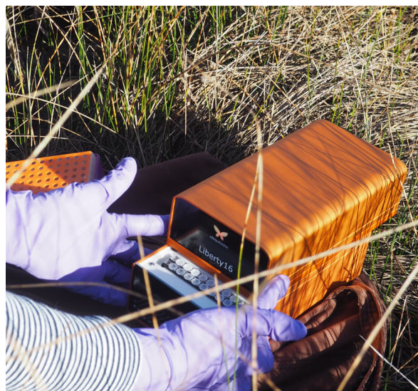
ABOVE: Handheld qPCR instrument that can detect DNA from target HAB species.
