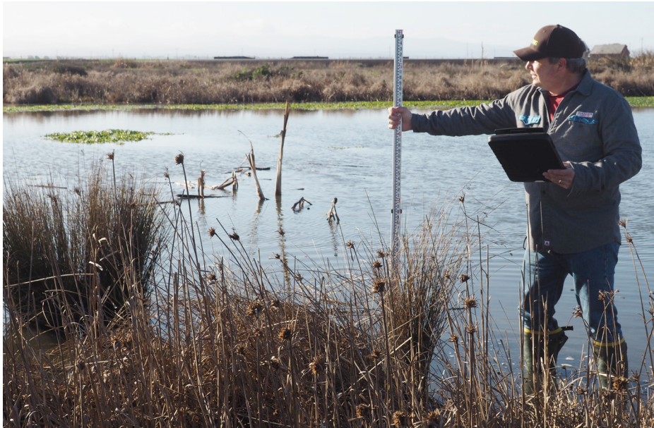
ABOVE: ABOVE: Ross Clark, Director of Central Coast Wetlands Group, SJSU Moss Landing Marine Labs, is taking water elevation stick measurements.
