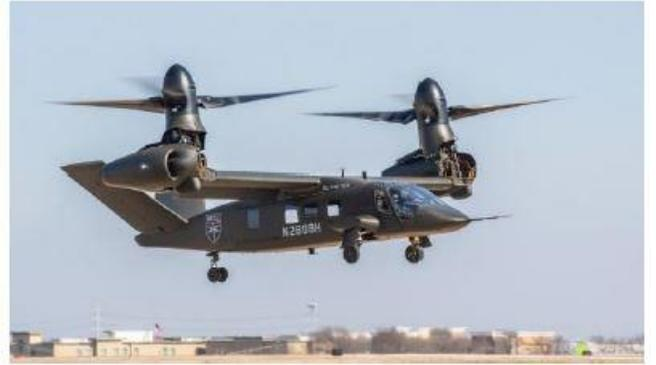
**Figure 2. V-280 in VTOL Mode flight.**
