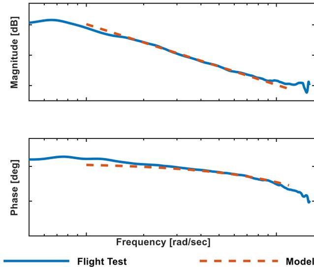
**Figure 12. DCP to roll rate frequency response from JIO and low order transfer function approximation.**
