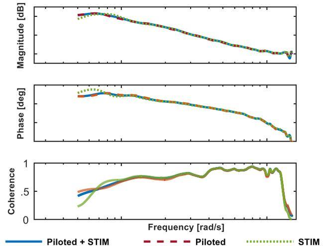
**Figure 8. Roll rate due to DCP frequency response for automated versus piloted frequency sweeps.**
