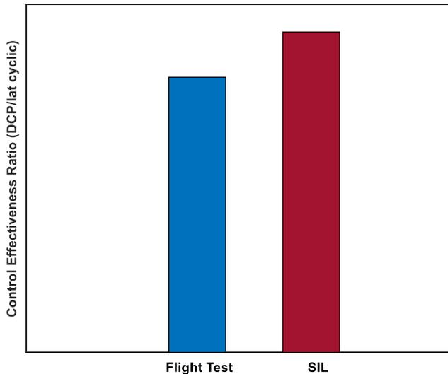
**Figure 17. Ratio of roll control effectiveness for DCP/(lateral cyclic).**
