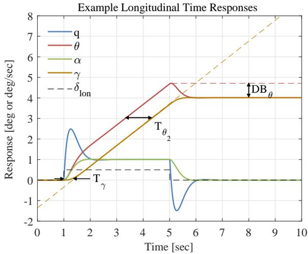
**Fig. 2. Example pitch attitude step response time history showing definition of flight path-attitude lag  $T_{\theta_2}$ , flight path lag  $T_{\gamma}$ , and pitch attitude dropback  $\text{DB}_{\theta}$ .**
