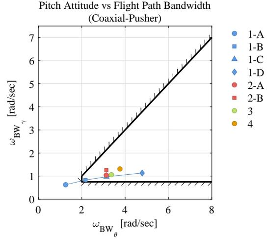
**Fig. 10. Flight path versus pitch attitude bandwidth values for command model variations (coaxial-pusher).**
