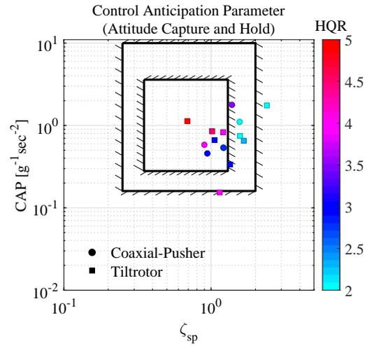
**Fig. 30. Pitch Attitude Capture and Hold handling qualities ratings plotted on the Control Anticipation Parameter (CAP) requirement (coaxial-pusher and tiltrotor).**
