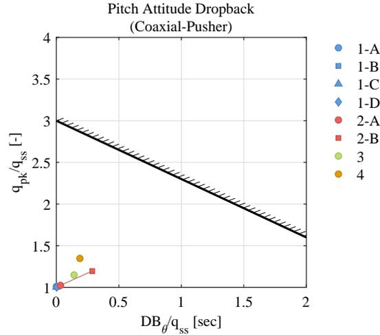
**Fig. 11. Pitch attitude dropback values for command model variations (coaxial-pusher).**
