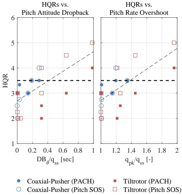
**Fig. 32. Handling qualities ratings plotted as a function of pitch attitude dropback and pitch rate overshoot (coaxial-pusher and tiltrotor)**
