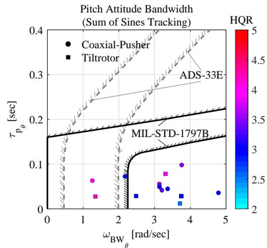
**Fig. 23. Pitch Sum-of-Sines Tracking handling qualities ratings plotted on the pitch attitude bandwidth requirement (coaxial-pusher and tiltrotor).**
