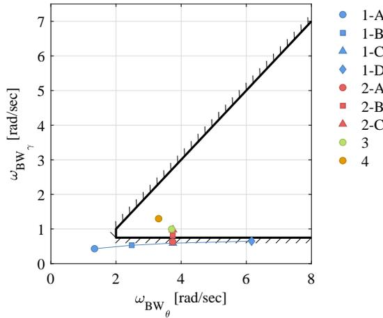
**Fig. 15. Flight path versus pitch attitude bandwidth values for command model variations (tiltrotor).**
