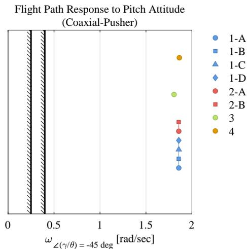
**Fig. 13. Flight path response to pitch attitude values for command model variations (coaxial-pusher).**
