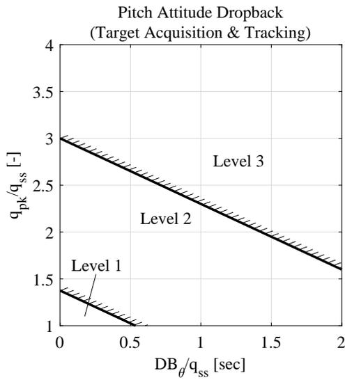
**Fig. 36. Proposed requirements for pitch attitude dropback – forward flight (Target Acquisition & Tracking).**
