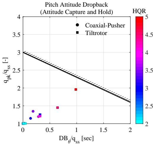
**Fig. 29. Pitch Attitude Capture and Hold handling qualities ratings plotted on the pitch attitude dropback requirement (coaxial-pusher and tiltrotor).**
