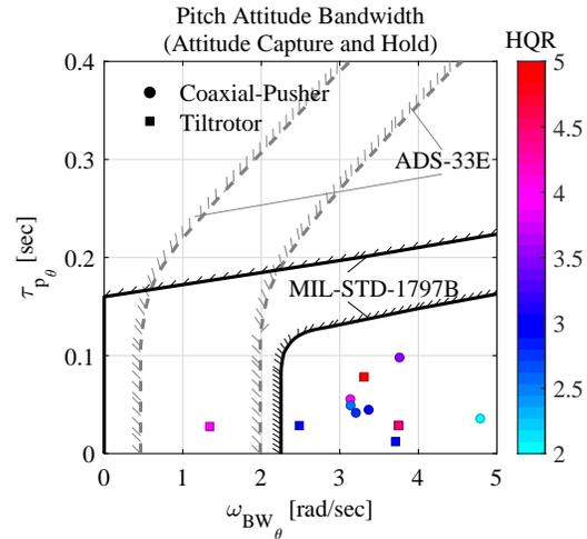
**Fig. 27. Pitch Attitude Capture and Hold handling qualities ratings plotted on the pitch attitude bandwidth requirement (coaxial-pusher and tiltrotor).**
