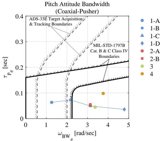
**Fig. 9. Pitch attitude bandwidth values for command model variations (coaxial-pusher).**
