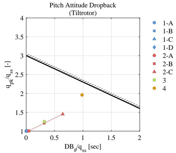
**Fig. 16. Pitch attitude dropback values for command model variations (tiltrotor).**
