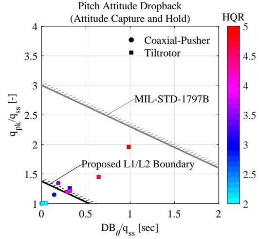
**Fig. 33. Pitch Attitude Capture and Hold handling qualities ratings plotted on the pitch attitude dropback requirement with proposed Level 1/Level 2 boundary (coaxial-pusher and tiltrotor).**
