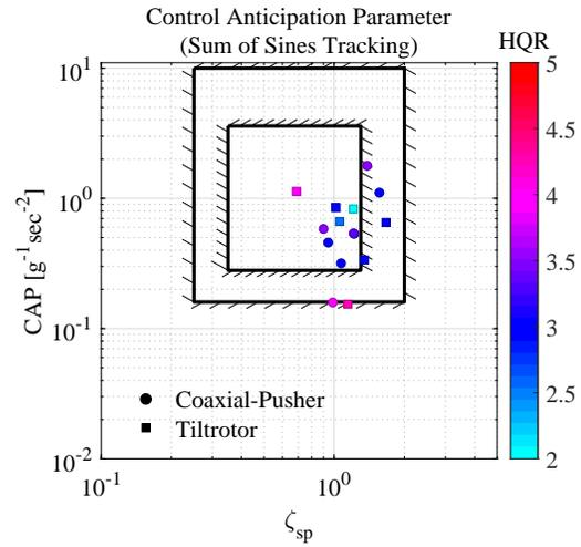
**Fig. 26. Pitch Sum-of-Sines Tracking handling qualities ratings plotted on the Control Anticipation Parameter (CAP) requirement (coaxial-pusher and tiltrotor).**
