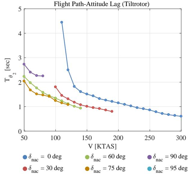
**Fig. 4. Bare-airframe flight path-attitude lag  $T_{\theta_2}$  values (tiltrotor).**
