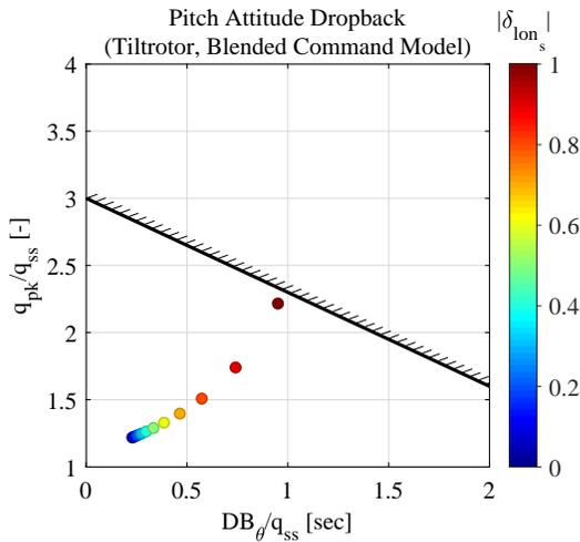
**Fig. 20. Pitch attitude dropback values for fight path rate blended command model (tiltrotor).**
