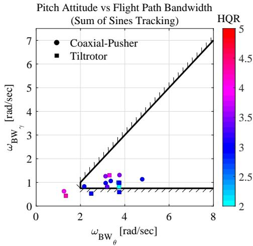
**Fig. 24. Pitch Sum-of-Sines Tracking handling qualities ratings plotted on the pitch attitude versus flight path bandwidth requirement (coaxial-pusher and tiltrotor).**
