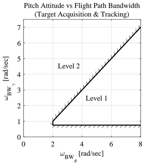
**Fig. 37. Proposed requirements for transient flight-path response (flight path bandwidth vs pitch attitude bandwidth) – forward flight (Target Acquisition & Tracking).**
