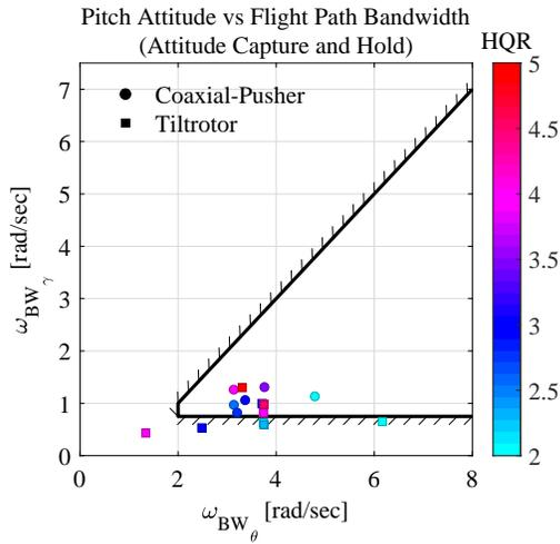
**Fig. 28. Pitch Attitude Capture and Hold handling qualities ratings plotted on the pitch attitude versus flight path bandwidth requirement (coaxial-pusher and tiltrotor).**
