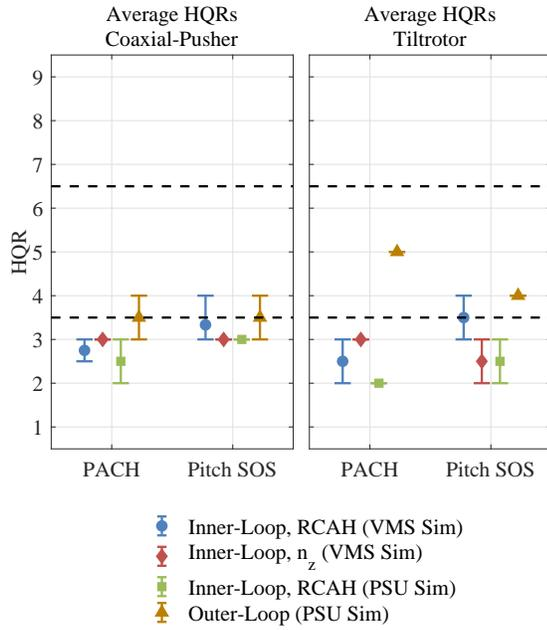
**Fig. 5. Previously collected pilot handling qualities ratings (HQRs) for inner- and outer-loop response types (coaxial-pusher and tiltrotor, Refs. 6 and 7).**
