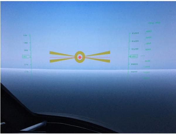
**Fig. 22. Display for Pitch Sum-of-Sines Tracking and Attitude Capture and Hold tasks.**
