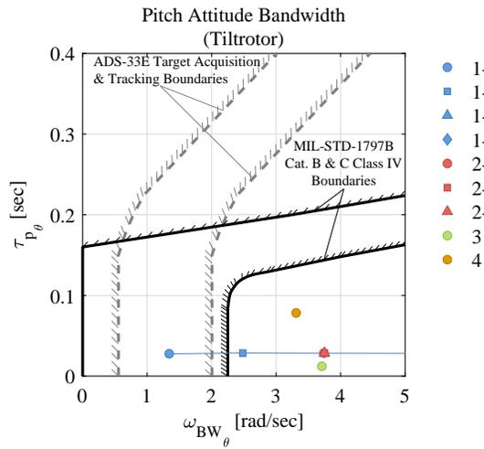
**Fig. 14. Pitch attitude bandwidth values for command model variations (tiltrotor).**
