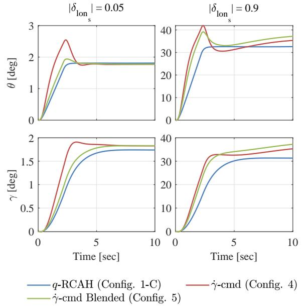
**Fig. 21. Pitch attitude and flight path response comparison for  $q$ -RCAH (Inner Loop, Configuration 1-C), flight path rate command (Outer Loop, Configuration 4), and flight path rate blended command model (Outer Loop, Configuration 5) (tiltrotor).**
