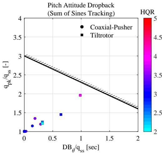
**Fig. 25. Pitch Sum-of-Sines Tracking handling qualities ratings plotted on the pitch attitude dropback requirement (coaxial-pusher and tiltrotor).**
