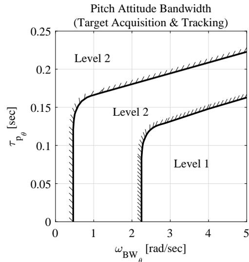
**Fig. 35. Proposed requirements for small-amplitude pitch attitude changes (pitch attitude bandwidth) – forward flight (Target Acquisition & Tracking).**
