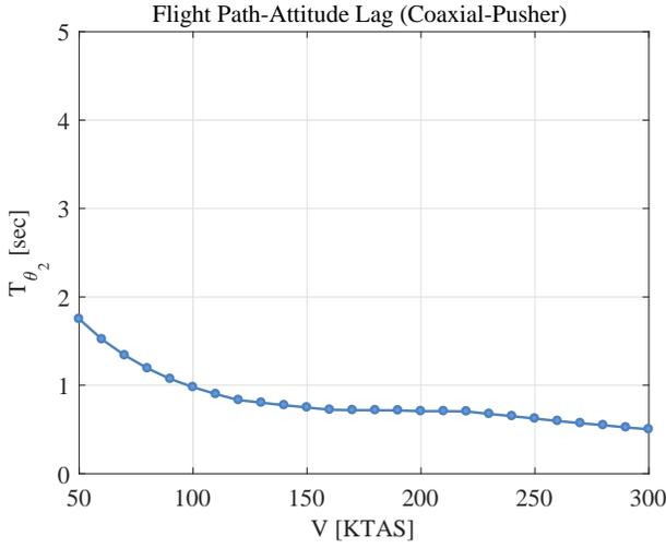
**Fig. 3. Bare-airframe flight path-attitude lag  $T_{\theta_2}$  values (coaxial-pusher).**
