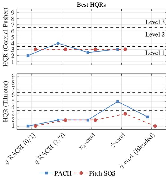
**Fig. 34. Lowest (best) pilot handling qualities ratings attained for each response type for the Pitch Attitude Capture and Hold and Pitch Sum-of-Sines Tracking tasks (coaxial-pusher and tiltrotor).**
