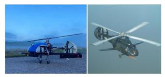
Figure 1. ADAPT<sup>TM</sup> Scaled Demonstrator (left) and X-49A (right) [2].
