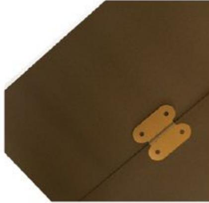
A simple hinge would allow the table top to freely move and collapse.
