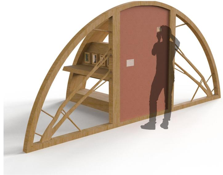
Cork surface would allow for multiple pinning and be replaceable when needed.
