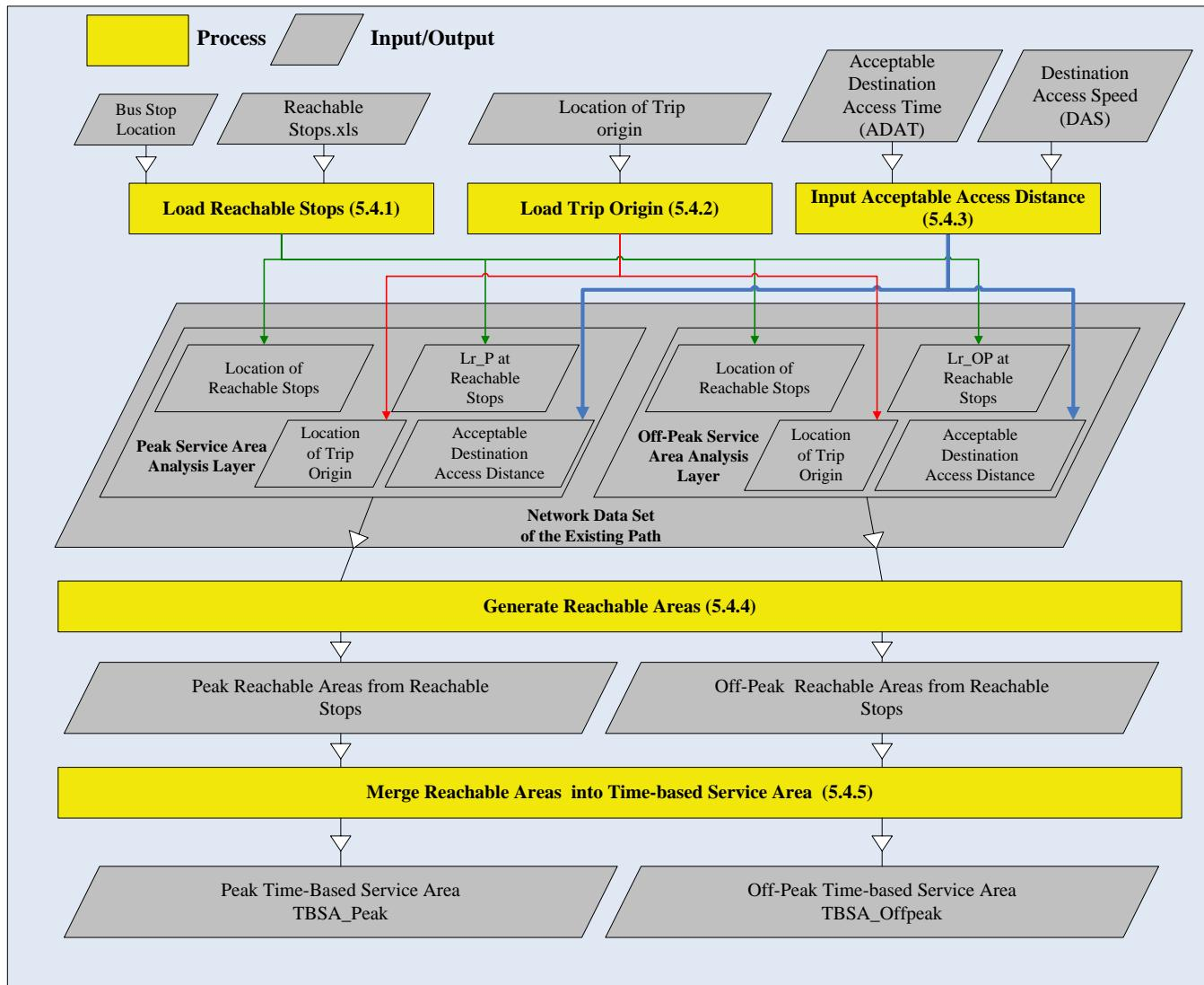
Figure 50: Phase 1 Process Flowchart: Find Accessible Bus Stops
