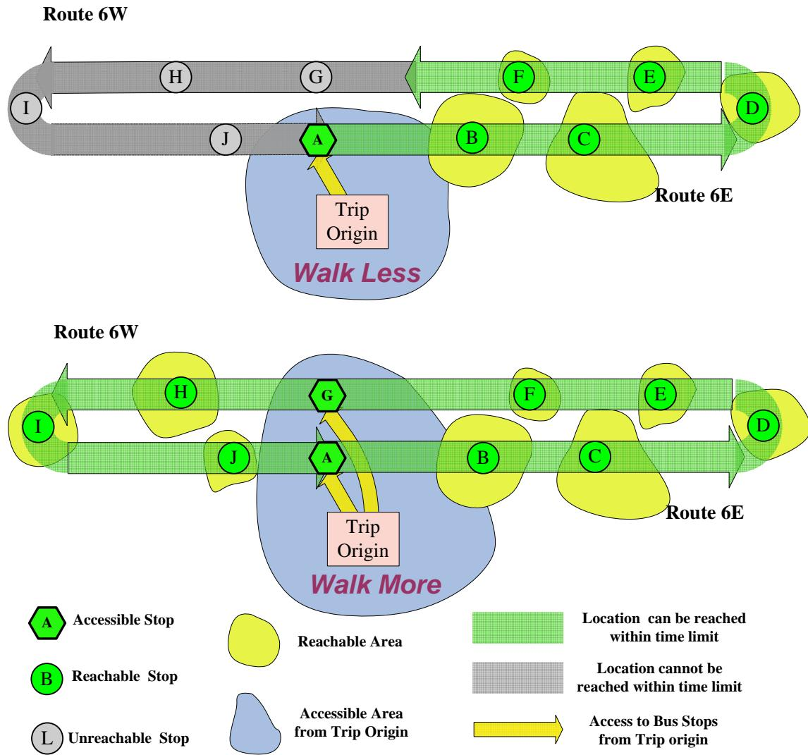
Figure 28: Reachable Stops Increases with Longer Walking Times
