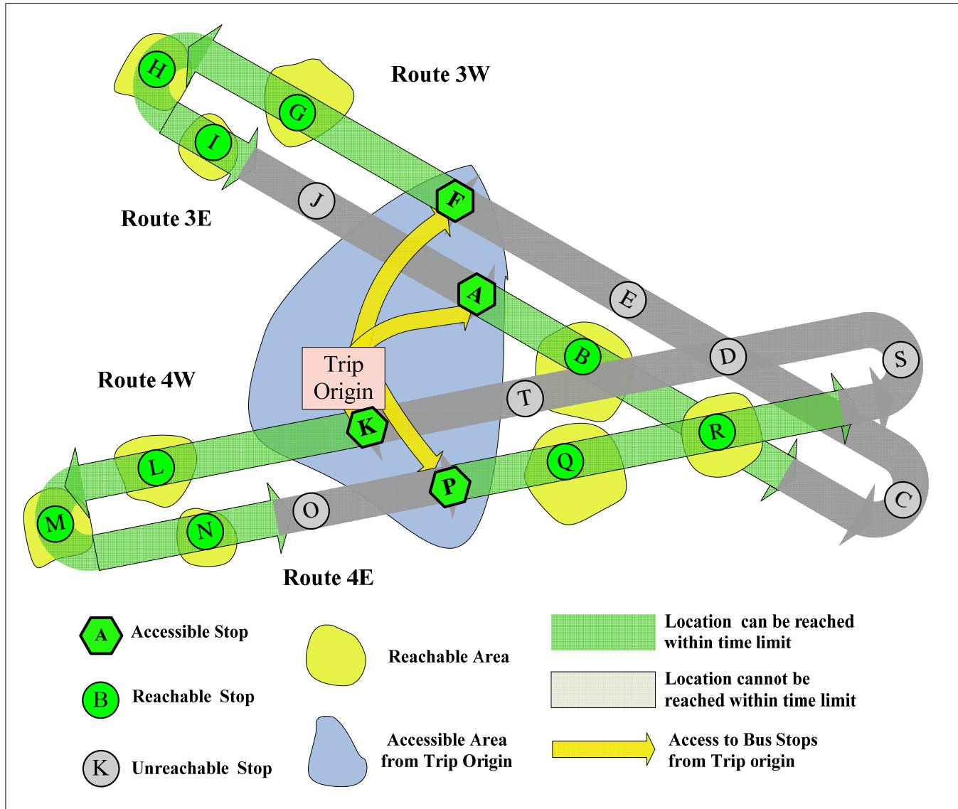
Figure 10: Multiple  $T_r$  Due to Reaching the Same Bus Stop through Different Routes
