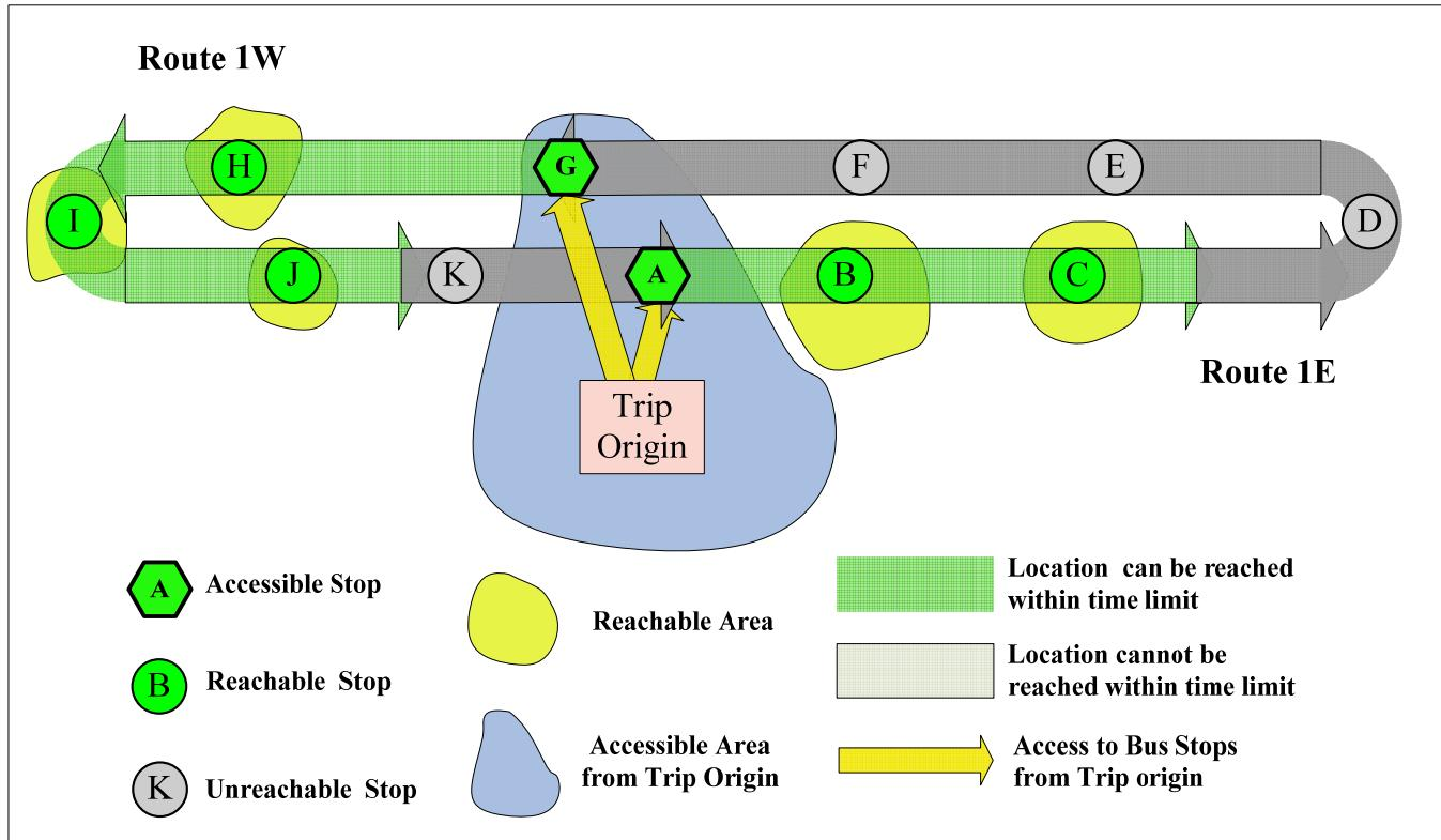
Figure 8: Diagram of Typical Time-Based Bus Service Area
