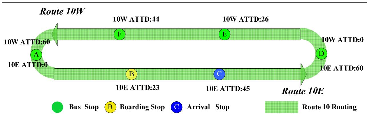
Figure 18: Calculate Bus travel Time (Type I)
