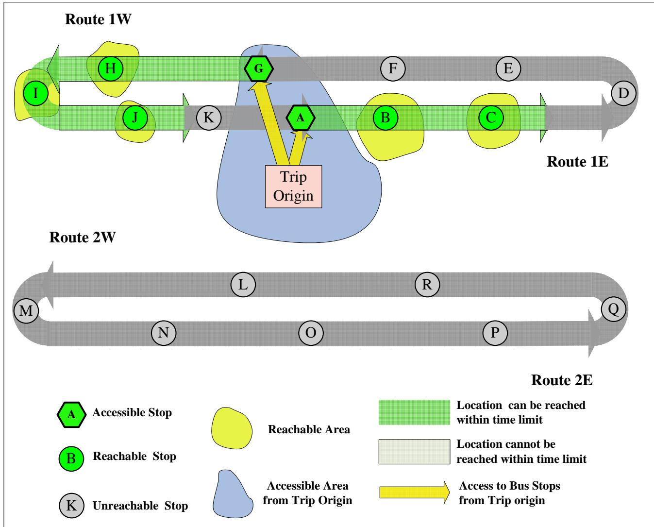
Figure 9: Accessible Route vs. Non-Accessible Route
