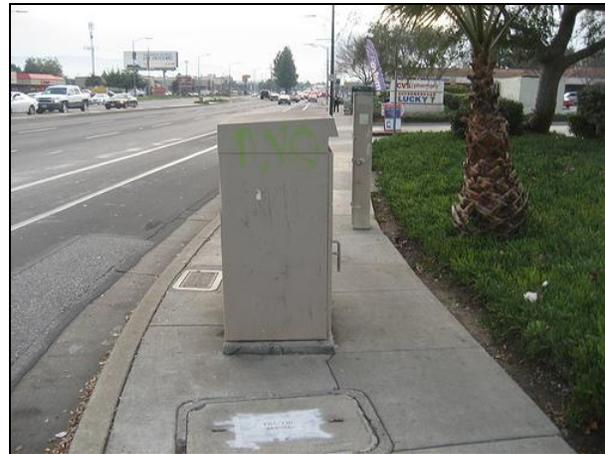
**Figure 36. Utility box obstruction near intersection.**
