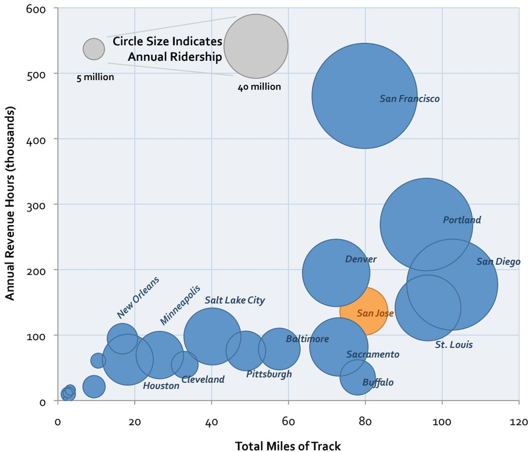
**Figure 9. Light Rail System Basics Peer Comparison**
