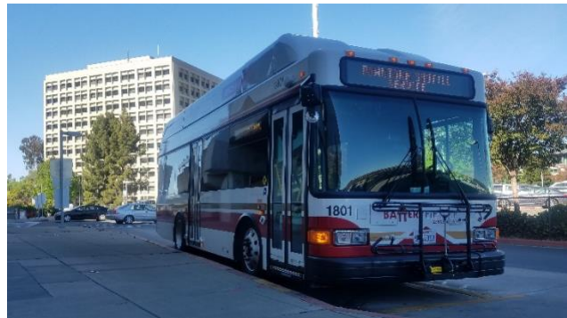
Figure 48: A Gillig 29-footer All-Electric Transit Bus with County Connection on layover at Walnut Creek BART. Marin Transit can emulate what the East Bay transit agency is doing to combat traffic by purchasing all-electric buses and offering free rides through generous subsidies.
