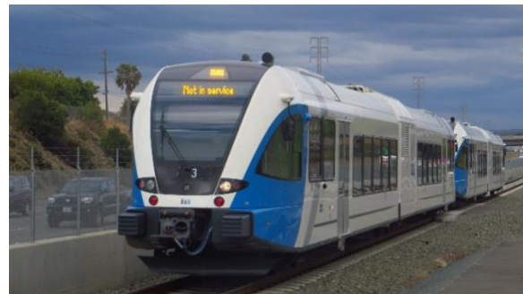
Figure 27: A 2-car Stadler GW2-6 train arriving at Pittsburg Center station on eBART (Eastern Costa Costa BART)
