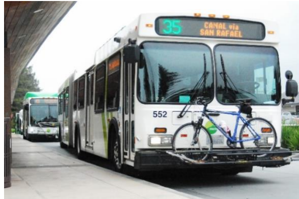
Figure 20: Two Marin Transit buses at Redwood & Grant in Downtown Novato: a New Flyer D60LF articulated bus operated by Golden Gate Transit on a southbound Route 35, and a Gillig BRT 40-footer Hybrid Bus operated by Marin Airporter on a southbound Route 49.
