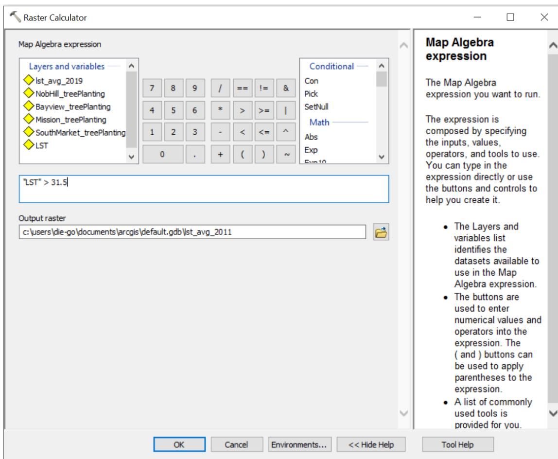
Figure 20: Raster Calculator Tool Used to Determine areas Above the Average Temperature of the Mission Neighborhood.
