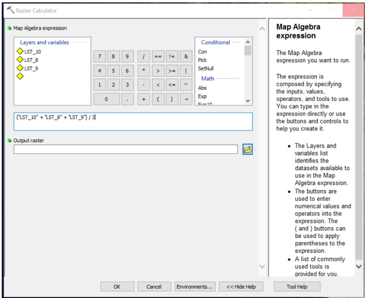
Figure 9: Raster Calculator Tool Averaging the LST Rasters for the Months of July, September, and October 2019. Source: Image created by author.
